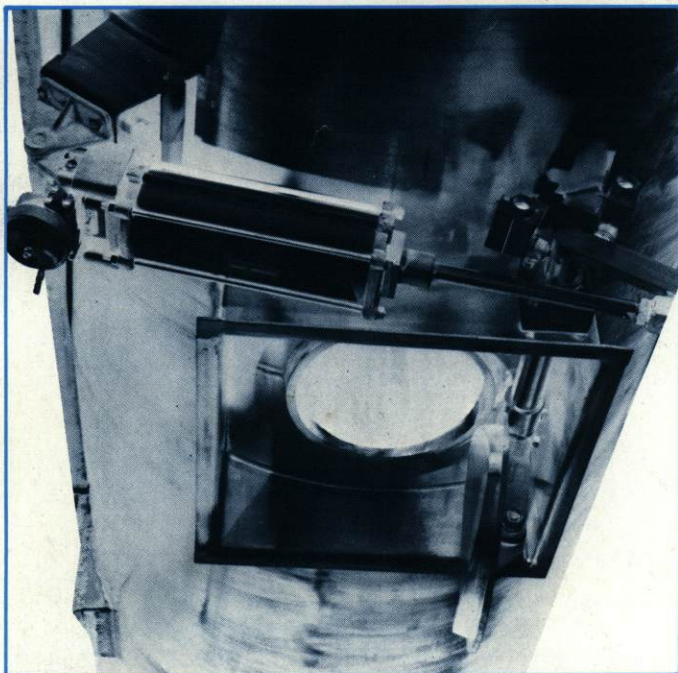
Optional pneumatic, contoured flush plug valve which allows remote operated discharge.
