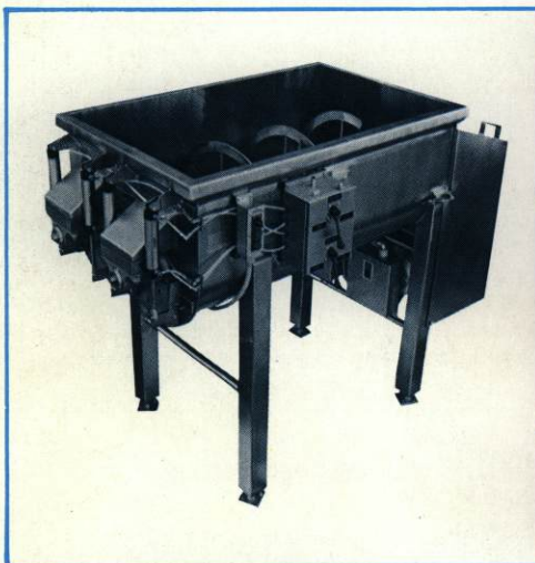
Single ribbon, twin agitator USDA approved meat blenders.
